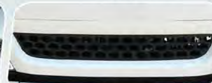
National pattern design with bigger radiator hole for better heat dissipation
