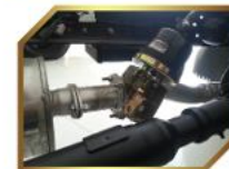
Extra Braking Efficiency with Exhaust Brake System
